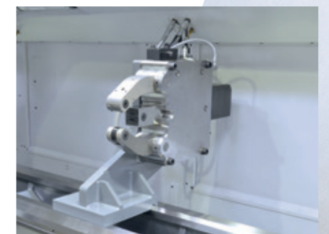
Steady rest, hydraulically actuated
