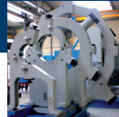
Steady rests for diameters up to 1,500 mm
