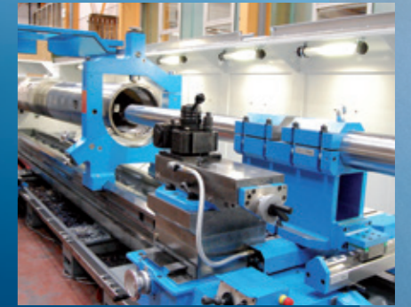
Heavy-duty boring bar holder with additional support and 160 mm bore
