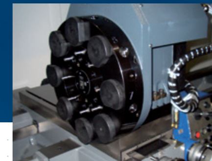
8 station disk turret with driven tools, 40 mm shank diameter
