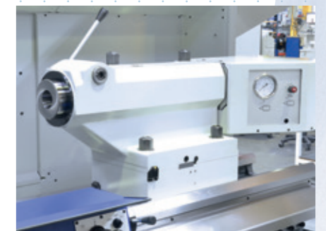
Tailstock with hydraulically actuated quill
