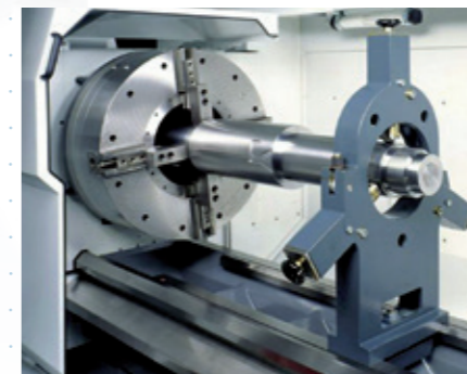
Pneumatically actuated front-end chuck with steady rest
