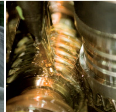
Gear wheel production / hobbing
